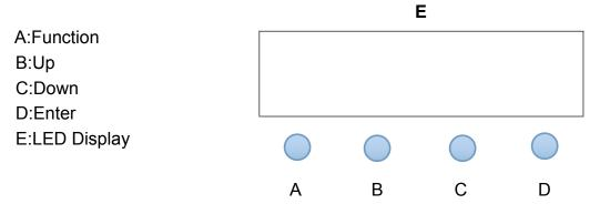
Instructions:Press the function key A cycled out the 13/19 different function effects, digital tube first two digits on behalf of which the current function (see menu). The last two digits represent the functions in which the address code or speed parameters. Press the B or C key to modify the parameter values. Press the D key to confirm.
