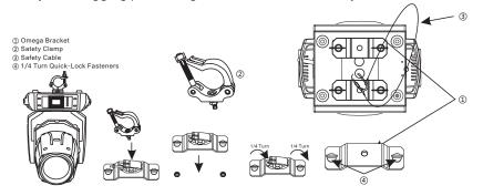
Regardless of the rigging option you choose for your JNR BWS 350, always be sure to secure your fixture with a safety cable. The fixture provides a built-in rigging point for a safety cable on the hanging bracket as illustrated above. Be sure to only use the designated rigging point for the safety cable and never secure a safety cable to a carrying handle.
