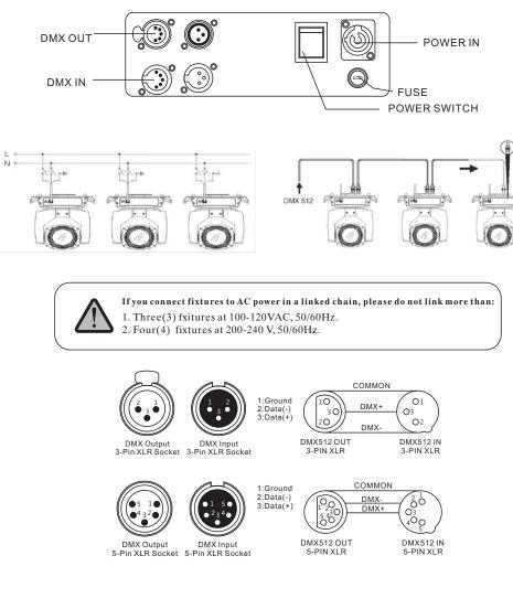
For installations where the DMX cable has to run a long distance or is in an electrically noisy environment, such as in a discotheque, it is recommended to use a DMX terminator. This helps in preventing corruption of the digital control signal by electrical noise. The DMX terminator is simply an XLR plug with a  $120 \Omega$  resistor connected between pins 2 and 3, which is then plugged into the output XLR socket of the last fixture in the chain. Please see illustrations below.
