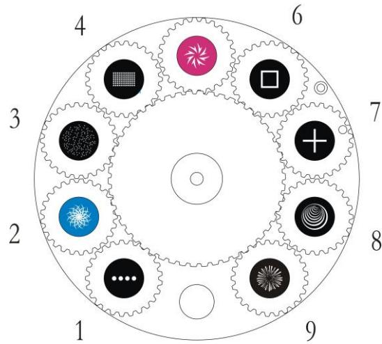
Two rotation prism, one 8 facet prism, one linear 4 prism, one fixed 16 prism,each two prism can combined using together. Frost function.
