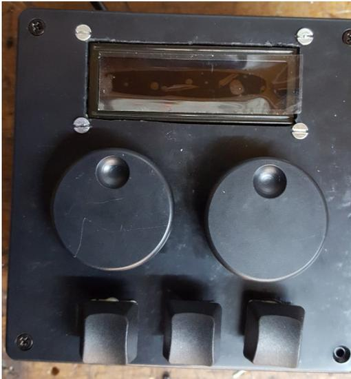
40. Secure the screen in place using eight #2-56 machine screws (four from the top, and four from the bottom) and either the  $\frac{1}{4}$ " (~6mm) or  $\frac{1}{2}$ " (~12mm) standoffs. Extra screws and standoffs are provided.
