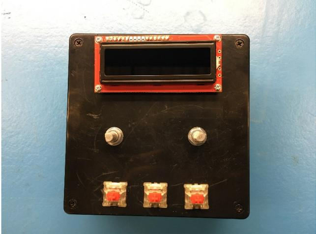
45. Press-fit the keycaps and encoder finger wheels onto the key switches and encoders.
