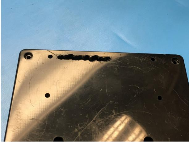
**TIP:** It may be helpful to trace the edges of the square holes into the plastic with an X-Acto knife, and then remove the paper.
