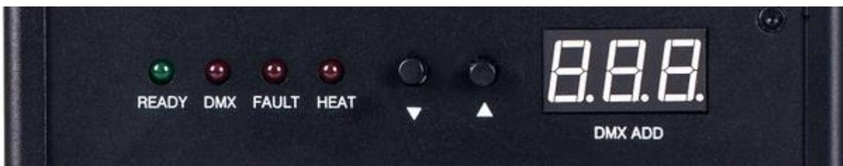
**READY:** After set the first channel(240-255 pre-heat ON) for about 5 minutes, when the "READY" green light turns from flash light to continuous light , it indicates that the machine is ready to work.
