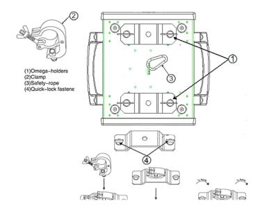
Regardless of the rigging option you choose for your SPOT LED, always be sure to secure your fixture with a safety cable. The fixture provides a built-in rigging point for a safety cable on the hanging bracket as illustrated above. Be sure to only use the designated rigging point for the safety cable and never secure a safety cable to a carrying handle.
