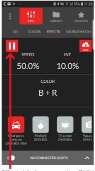
Effect Mode: press the PLAY button, select the effect, change speed, instensity and the color of the LEDs.
