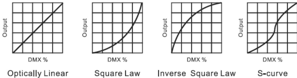
**Linearity:** As the DMX value increases, the increase in light intensity tends to be linear
