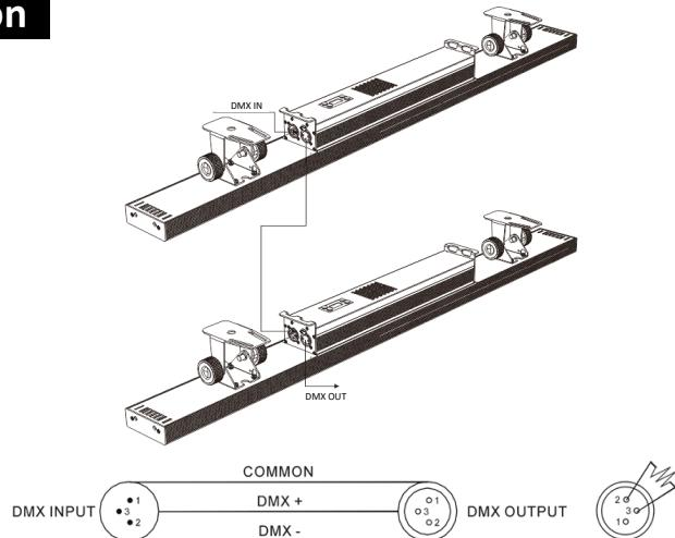
1. At last unit, the DMX cable has to be terminated with a terminator. Solder a 120-ohm 1/4W resistor between pin 2(DMX-) and pin 3(DMX+) into a 3-pin XLR-plug and plug it in the DMX-output of the last unit.
