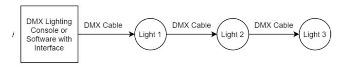
**32 Fixture Rule** – DMX only allows you to connect up to 32 fixtures in a single daisy chain for signal strength. Sometimes, depending on the fixtures and cable length, this number is less (or more).
