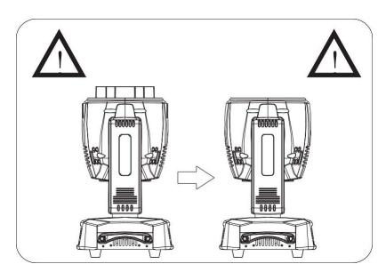
Before packing, let the head lens retract, or the lens will be destroyed in transportation.
