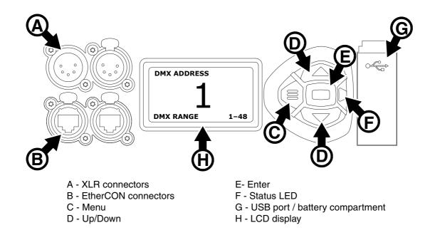
Figure 5: Display and control panel
