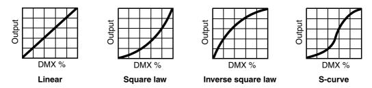
Figure 6: Dimming curve options
