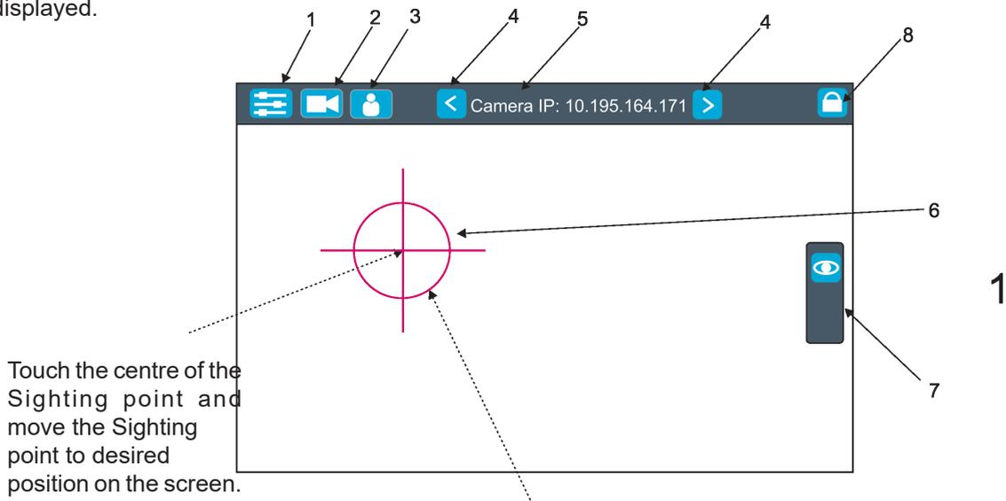
Touch the centre of the Sighting point and move the Sighting point to desired position on the screen.
