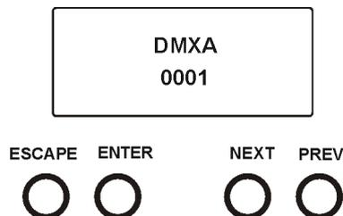
After switching the fixture on, display shows current DMX address.
