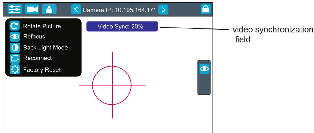
Rotate Picture- use this item to rotate a picture on the touch screen 180 degrees from current orientation.
