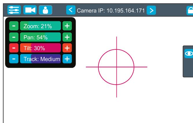
Camera Zoom slider- use it to change a zoom of currently selected camera. A sensitivity of a camera zoom can be set in three levels: low (green slider), medium (yellow slider) and high (red slider).
