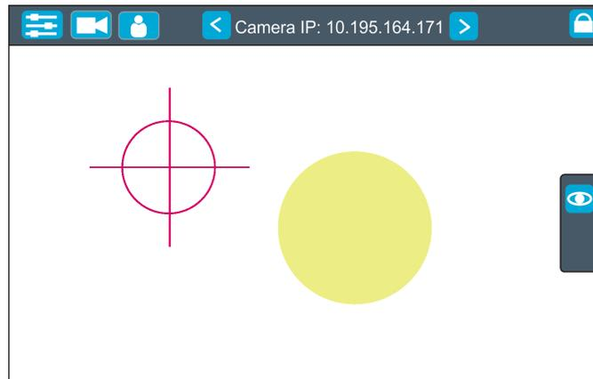
3. Move the sighting point on the beam image. Now, when you move with the control handlebars, both beam image and sighting point on the screen will move synchronously. It is useful in case that the light output from the fixture is closed and by means of the sighting point you approximately know the position of the light beam.
