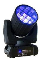
This Led light is designed to create beam flower effects using RGBW Leds either as stand alone or DMX controlled with either 18 or 29 DMX channels with DMX input and output on 3 pin XLR connectors.
