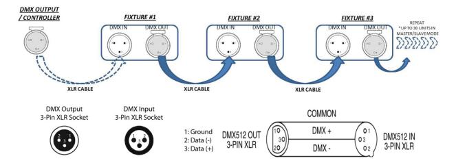
For installations where the DMX cable has to run for a long distance, or as an electrically noisy environment, it is recommended to use a DMX terminator. This helps in preventing corruption of the digital control signal by electrical noise. The DMX terminator is simply an XLR plug with a 120 resistor connected between pins two and three, which is then plugged into the output XLR socket of the last fixture in the chain.
