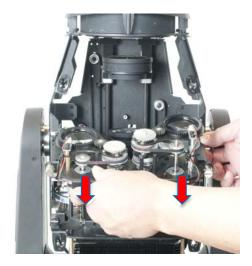
4. Optional. This step may be performed to help improve access to the gobo wheel module. Loosen the thumb screws for the prism module, and carefully slide the prism module out of its mounting slots. Set the prism module aside for later reinstallation.
