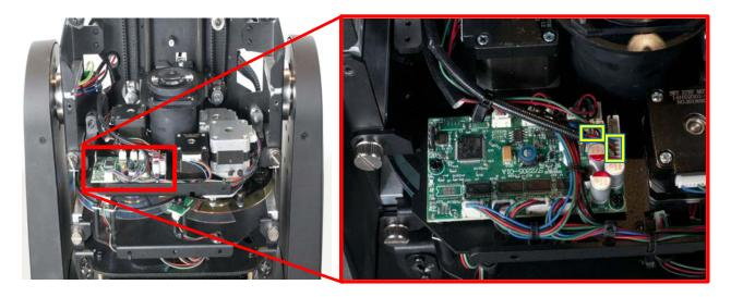
5. On the gobo wheel module, locate the circuit board on the left hand side of the gobo wheel module, directly above the static gobo wheel. On this circuit board, find the 3-pin connector and the 4-pin connector (denoted by the yellow boxes, above right) located just behind a bank of three (3) capacitors, and disconnect both of these connectors.
