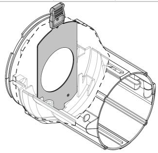
2. Insert the Soft edge filter into the slot. NOTE: To remove the accessory, reverse the procedure.
