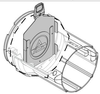
2. Insert the gobo holder into the slot. The flaps will go into the appropriate size. NOTE: To remove the accessory, reverse the procedure.
