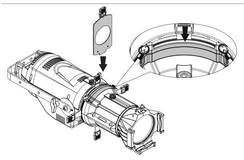
1. Loosen the marked screws. Then open the slot of the middle part.
