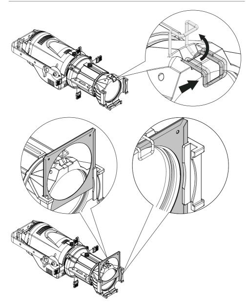
Push the clip, located at the top of the optics body, outwards and lift it. Then insert the filter into the marked track and close the clip, always applying an outward push.
