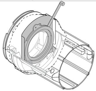
2. Insert the steel iris diaphram into the slot. The flaps will go into the appropriate size. NOTE: To remove the accessory, reverse the procedure.
