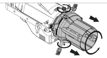
1. Loosen the marked knob and screw. Then rotate the middle part and remove it.
