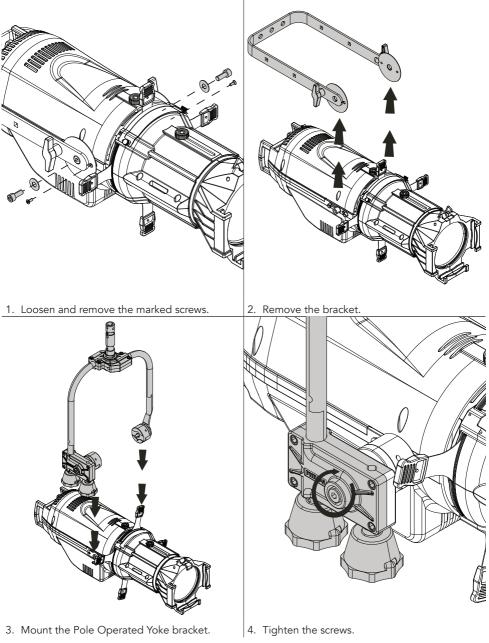
NOTE: To remove the accessory, reverse the procedure.
