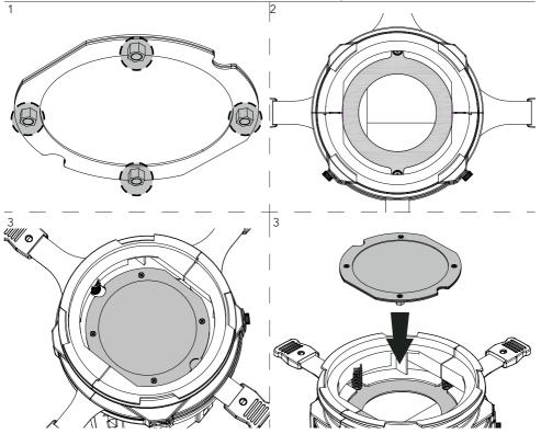
2. Insert the soft focus diffusion kit by placing the magnets (1) on the back of the framing system (2) of the middle part.
