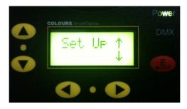
There are 13 sub-menus in the Setup Menu which give information and other data about the configuration and the status of Evolight fixture.
