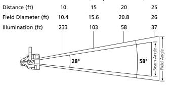
For Field diameter at any distance, multiply distance by 1.04. For Beam diameter at any distance, multiply distance by 0.50.
